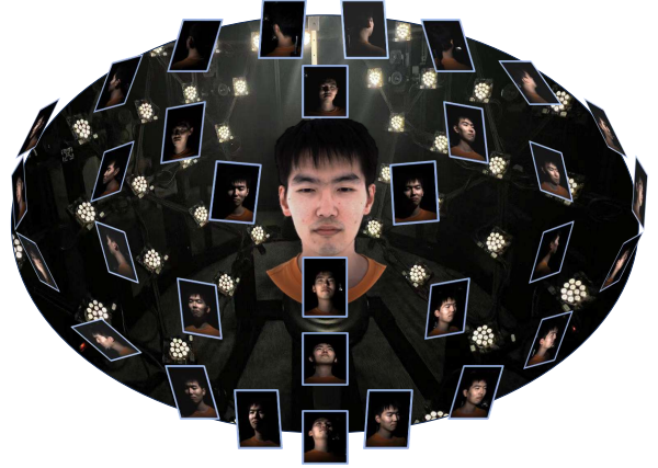
Figure 3. Our Light Stage consists of 156 LEDs and 32 synchronized cameras uniformly covering the full sphere. Each light is sequentially activated to produce OLAT captures.
